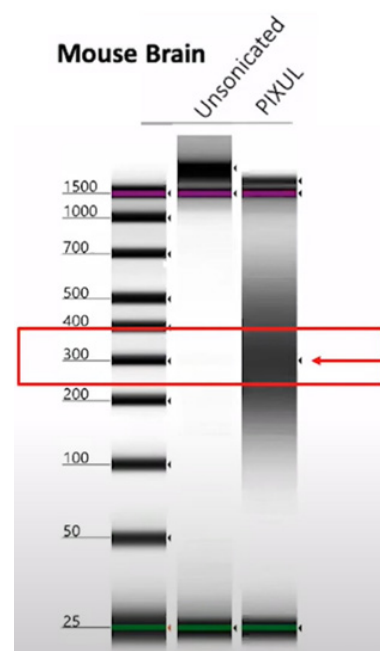
Figure 4: PIXUL-sonicated (Y) and unsonicated (N) chromatin purified from an input prep using mouse brain sample, analyzed on the Agilent 4200 TapeStation system.
