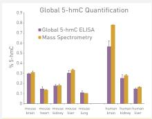
Figure 2: The Global 5-hmC Quantification Kit was used to determine the % 5-hmC in genomic DNA isolated from mouse and human tissues. Genomic DNA was tested at 20 ng/well for human brain and 50 ng/well for all other DNA samples. The % 5-hmC was determined using the included DNA standards. Results were compared to mass spectrometry data obtained from 500 ng of the same DNA samples. Results show the Global 5-hmC Kit provides equivalent quantification using only a fraction of the starting material.
