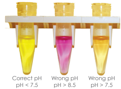
▲ FIGURE: The DNA Purification Binding Buffer has a pH indicator dye so the pH of the solution can be easily determined.
